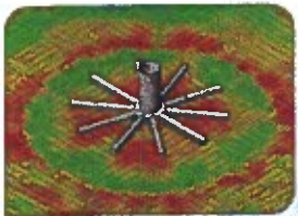
High horizontal velocity of water aids in sludge reduction
